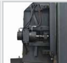
Hydraulic Blade Tension
