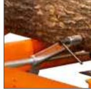
**Manual log clamp** for precisely clamping cants and the last board.
